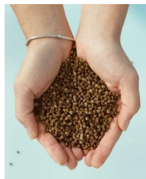
Bio-composite formulation from hop waste residues
